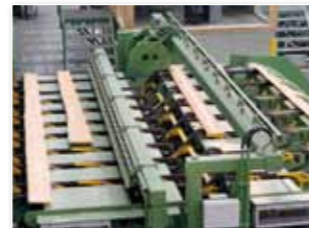
Board assessment area with stop hooks
