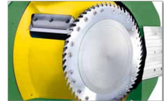
Straight knife chipper head with pre-sawing circular saw ring
