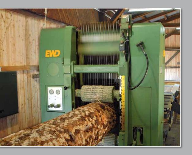
Cost-efficient sash gang for the use in small to medium-sized sawmills
