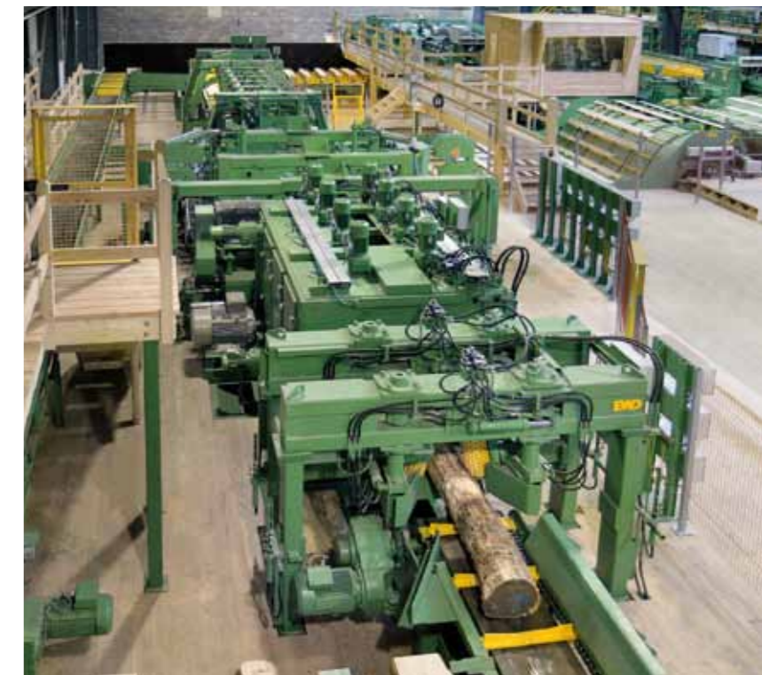
Medium production reducer saw line with double arbor circular saw DWK
