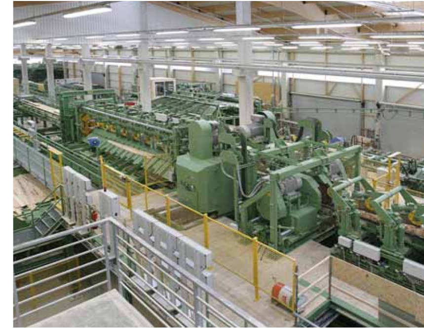
High production reducer saw line with double arbor circular saw DWK
